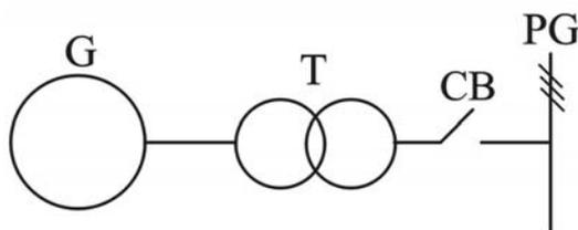
Fig.1. Power unit circuit: G – synchronous generator, T – transformer, CB – circuit breaker, PG – power grid
