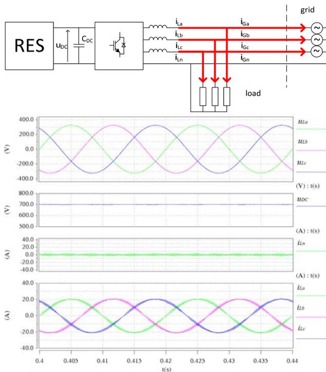
Fig.11. Grid-connected operation mode. From the top: load voltages  $u_{La}$ ,  $u_{Lb}$ ,  $u_{Lc}$ , DC-link voltage  $U_{DC}$ , neutral current  $i_{Ln}$ , converter currents  $i_{La}$ ,  $i_{Lb}$ ,  $i_{Lc}$
