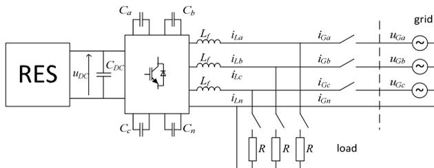
Fig.8. Three-phase four-leg three-level flying capacitor converter
