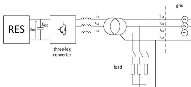
Fig.1. RES connected to the grid by three-phase three-leg converter with *dy* transformer.
