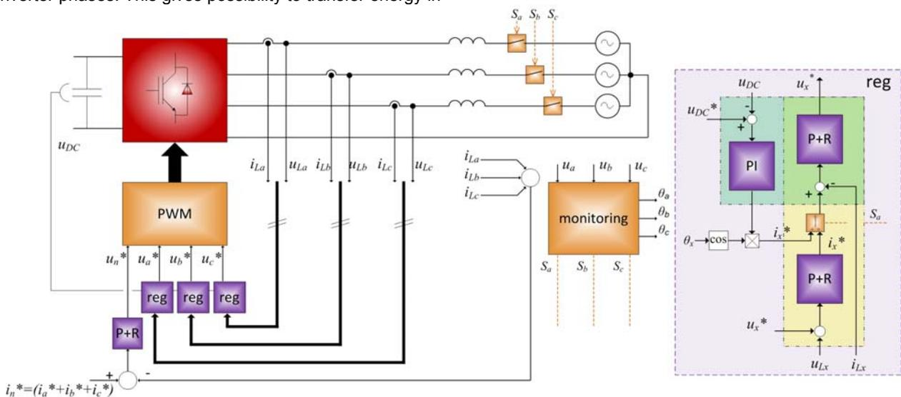
Fig.7. Block scheme of control method with P+R controllers
