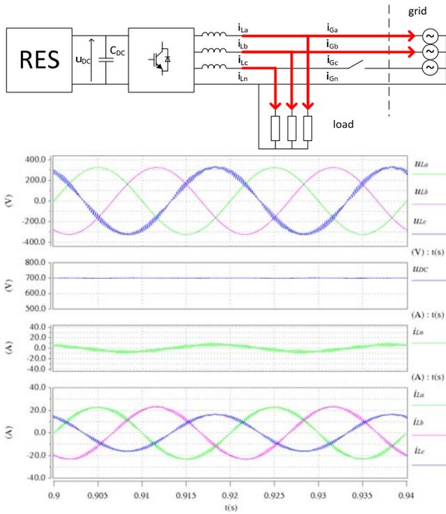
Fig.12. Mixed mode, grid without one phase. From the top: load voltages  $u_{La}$ ,  $u_{Lb}$ ,  $u_{Lc}$ , DC-link voltage  $U_{DC}$ , neutral current  $i_{Ln}$ , converter currents  $i_{La}$ ,  $i_{Lb}$ ,  $i_{Lc}$
