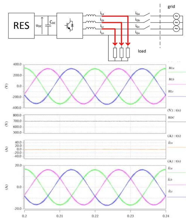
Fig.9 Stand-alone mode of operation. From the top: load voltages  $u_{La}$ ,  $u_{Lb}$ ,  $u_{Lc}$ , DC-link voltage  $U_{DC}$ , neutral current  $i_{Ln}$ , load currents  $i_{La}$ ,  $i_{Lb}$ ,  $i_{Lc}$
