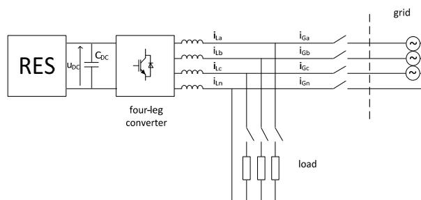
Fig.2. RES connected to the grid by three-phase four-leg converter.
