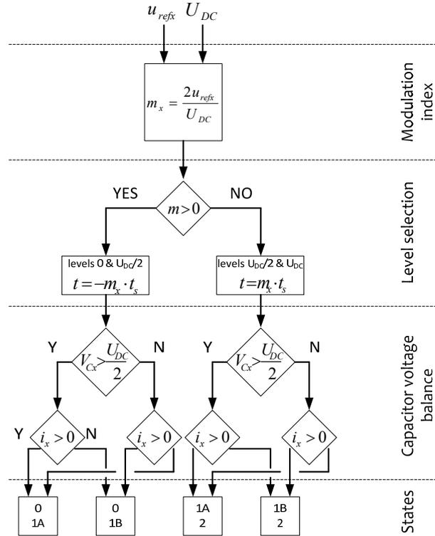
Fig.4. Signal flow diagram of 1DM for three-level flying capacitor converter
