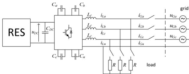
Fig.8. Three-phase four-leg three-level flying capacitor converter
