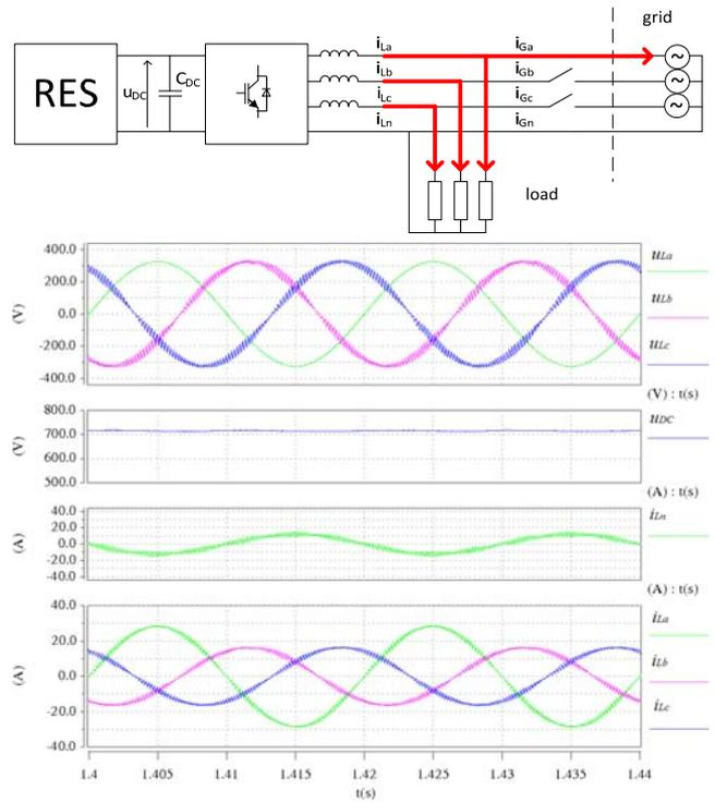
Fig.13. Mixed mode, grid without two phases. From the top: load voltages  $u_{La}$ ,  $u_{Lb}$ ,  $u_{Lc}$ , DC-link voltage  $U_{DC}$ , neutral current  $i_{Ln}$ , converter currents  $i_{La}$ ,  $i_{Lb}$ ,  $i_{Lc}$
