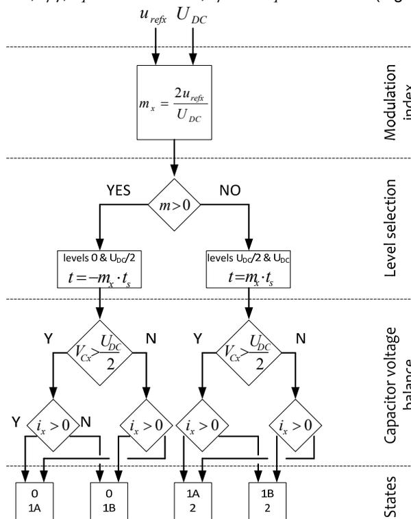
Fig.4. Signal flow diagram of 1DM for three-level flying capacitor converter
