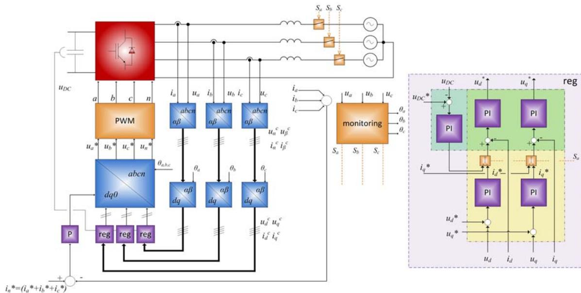
Fig.6. Block scheme of control method with PI controllers
