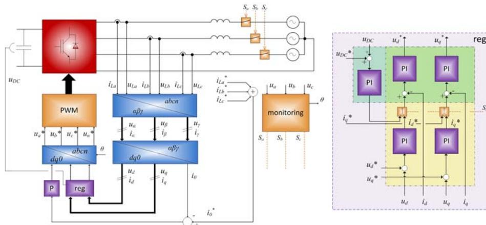
Fig.5. Block scheme of classical voltage oriented control method for four-leg converter with PI controllers
