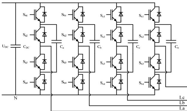
Fig.3. Three-level four-leg flying capacitor converter
