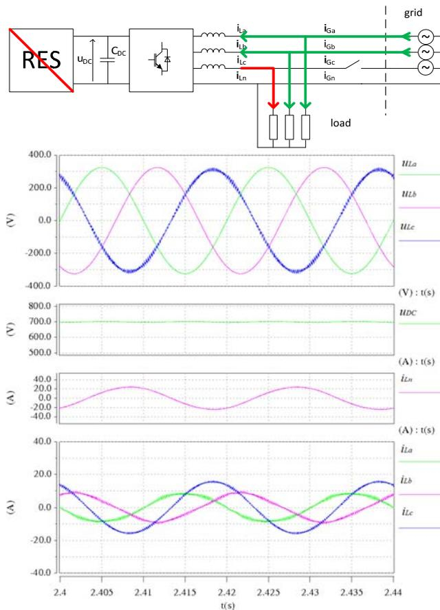
Fig.14. Mixed mode, grid without one phase and without RES. From the top: load voltages  $u_{La}$ ,  $u_{Lb}$ ,  $u_{Lc}$ , DC-link voltage  $U_{DC}$ , neutral current  $i_{Ln}$ , converter currents  $i_{La}$ ,  $i_{Lb}$ ,  $i_{Lc}$
