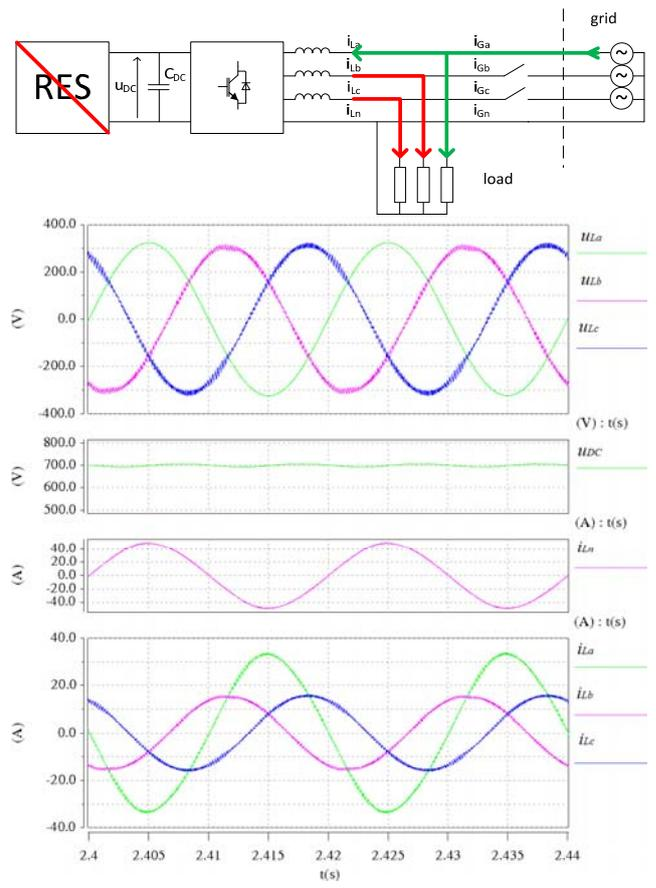
Fig.15. Mixed mode, grid without two phases and without RES. From the top: load voltages  $u_{La}$ ,  $u_{Lb}$ ,  $u_{Lc}$ , DC-link voltage  $U_{DC}$ , neutral current  $i_{Ln}$ , converter currents  $i_{La}$ ,  $i_{Lb}$ ,  $i_{Lc}$
