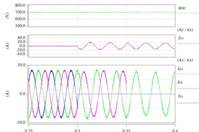
Fig.10. Stand-alone mode of operation. From the top: DC-link voltage  $U_{DC}$ , neutral current  $i_{Ln}$ , load currents  $i_{La}$ ,  $i_{Lb}$ ,  $i_{Lc}$
