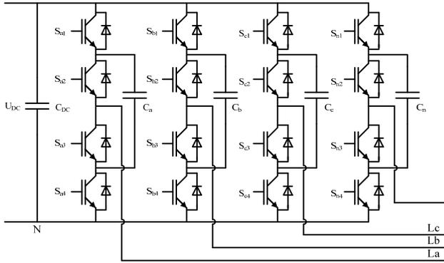
Fig.3. Three-level four-leg flying capacitor converter
