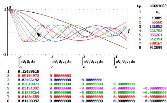
Fig. 15. First screen of program MECH, with finding eigen functions
