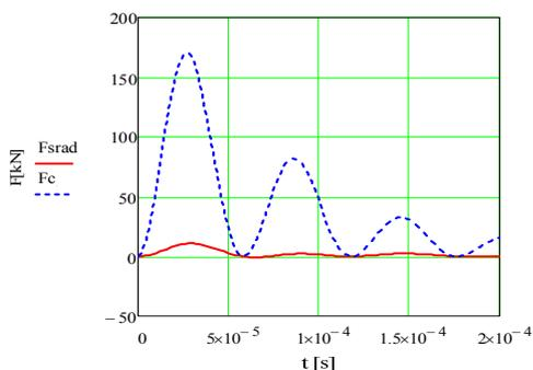
Fig. 12. Comparison of total radial and axial forces acting on the disc
