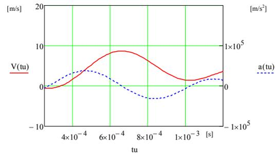
Fig.10. Trajectories  $v(t)$  and  $a(t)$  after differentiation  $x(t)$
