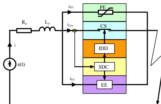
Fig.2. Block diagram of HCB in short circuit
