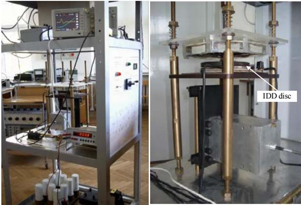
Fig.3. The measuring system and optimeter connected with IDD
