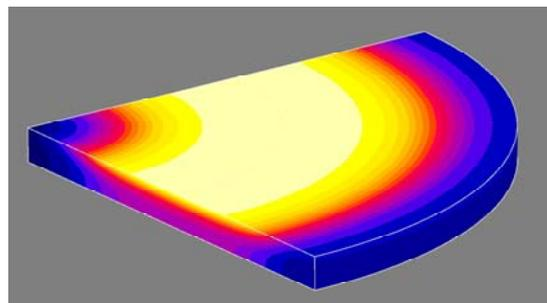
Fig. 13. Current distribution of disc in Flux program
