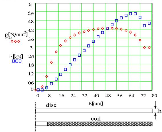
Fig.18. Distribution of pressure and force
