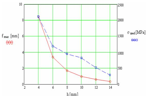
Fig.17. Results of maximal  $\sigma_{zr}$  and deflection for various thickness of the disc
