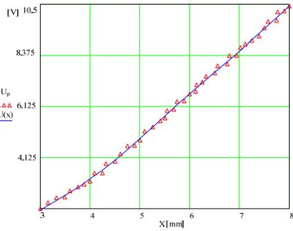
Fig.7. The output approximated characteristic -U(x)
