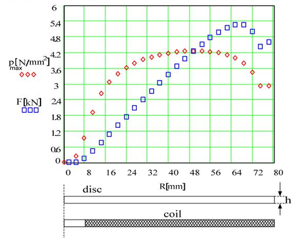
Fig.18. Distribution of pressure and force
