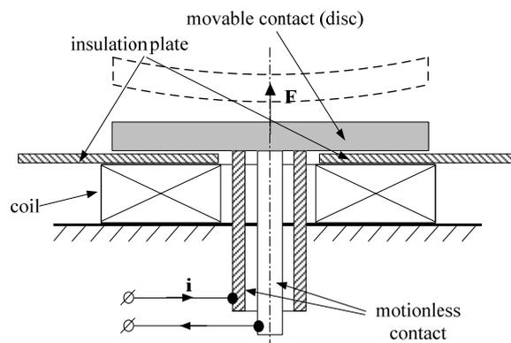
Fig.1. Construction of contact-IDD system and deformation of disc
