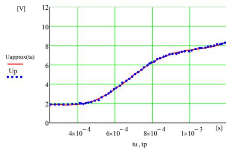
Fig.9. The voltage trajectory on the sensor terminals and its approximation
