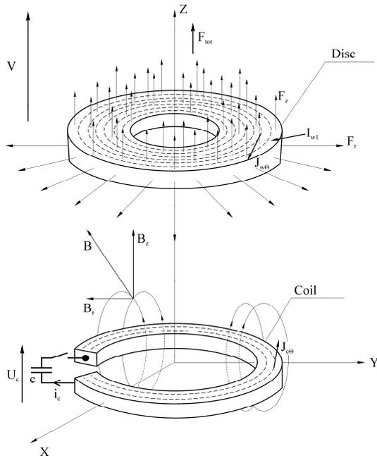
Fig. 11. Forces acting on the disc
