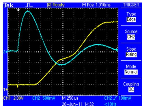
Fig.6. The oscillogram of the disc displacement and the coil current
