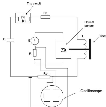
Fig.5. The measurement system to examine the coil current and the disc displacement
