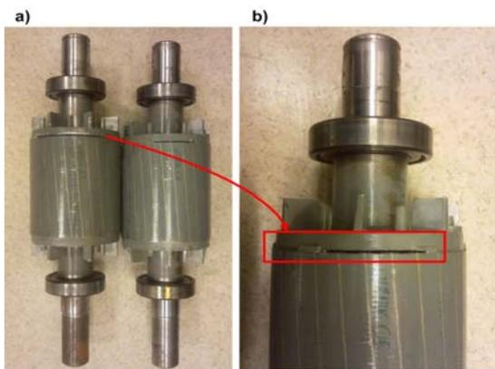
Fig.2. Rotors with different number of broken bars (8 and 4) (a) and zoom of the 8 broken rotor bars (b) prepared using spark erosion machine
