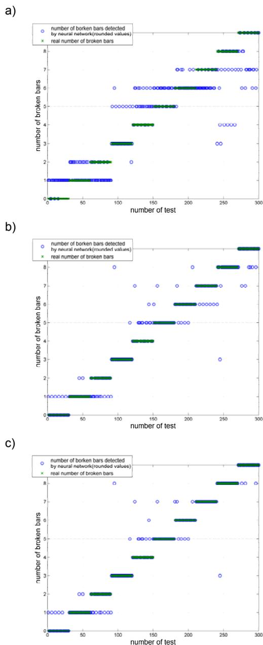
Fig.4. Graphical presentation of GRNN detector results for data set 4 and chosen  $\sigma$  values (for testing data): (a –  $\sigma = 0.5$ , b –  $\sigma = 0.1$ , c –  $\sigma = 0.05$ ); rounded values
