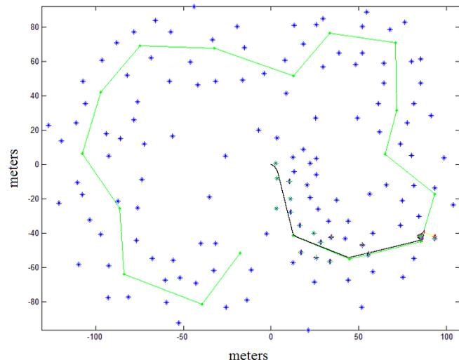
Fig. 4. EKF-based SLAM simulations used to evaluate the effect of vehicle speed on ATE
