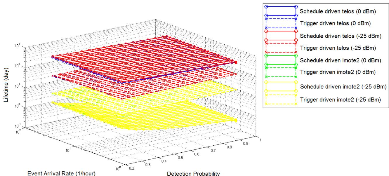
Fig. 2. Lifetime performances of imote2 and telos nodes for 0 dBm and -25 dBm transmit powers for schedule-driven and trigger-driven operating models
