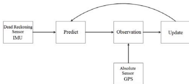
Fig. 3. GPS and IMU integrated EKF based localization and navigation system
