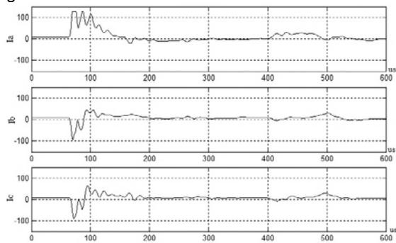
Fig.6. The recorded current travelling wave signals at Yafeng
