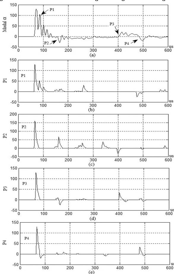
Fig.7. Fault travelling wave aerial mode component and constructed waveforms
