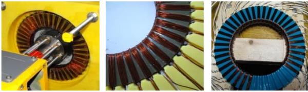
Fig. 1. (a) Left: Stator with multilayer windings (MLW); (b) Center: Stator with one-layer windings; (c) Right: Stator with slotted torus.
