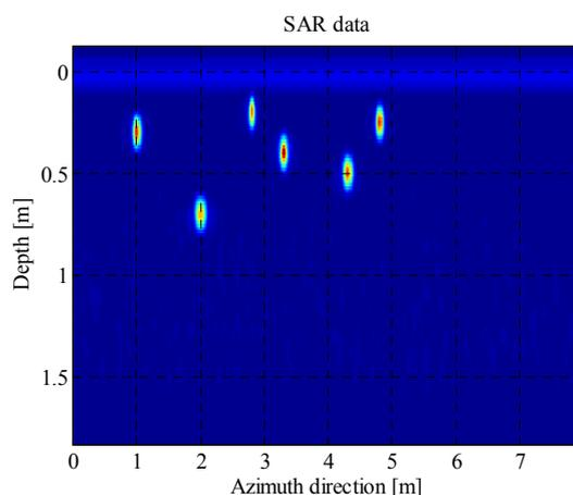
Fig.5. Fully focused SAR data.
