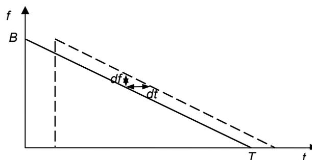
Fig.1. FMCW modulation function.
