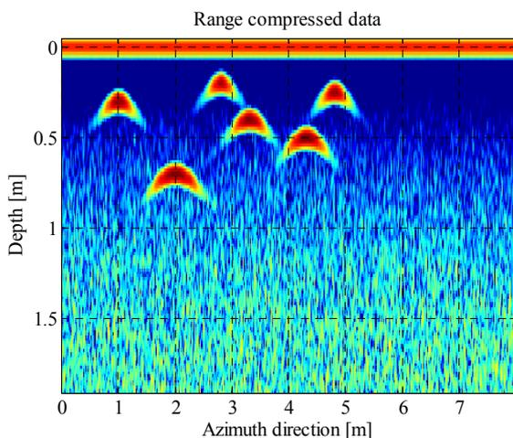
Fig.3. GPR range compressed data.
