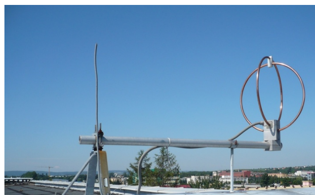
Fig. 2. The first LINET antenna installed in Poland in 2006 [7] working as a reference point of the lightning location system will be used for measurements of lightning magnetic field component. This year, new antennas shown in Fig. 1 and the FVC Photron SA5 shown in Fig. 3 will be mounted at the same roof together with the LINET sensor.
