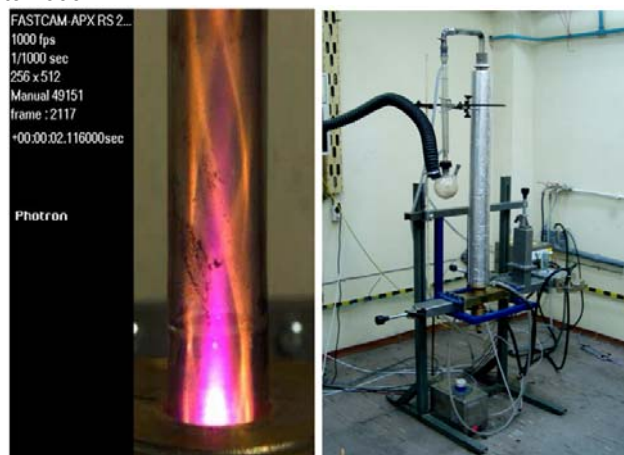
Fig. 1. The microwave plasma – left and the setup for synthesis of carbon nanotubes- right
