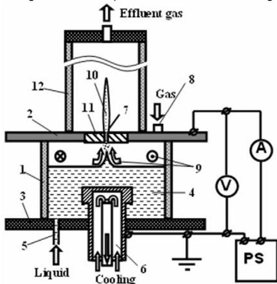
Fig.4. Schematic of the PLS reactor with the DC discharge in a reverse vortex gas flow of tornado type with a "liquid" electrode.
