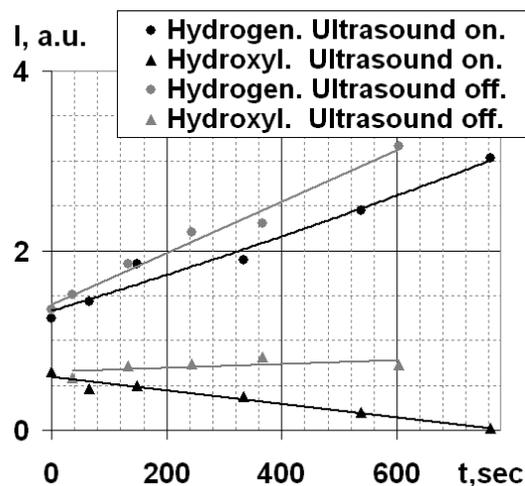
Fig.5. Dependences of the relative intensity of the hydroxyl molecular band – trigonal points and hydrogen – round points in the emission spectra of DGCLW plasma on the distilled water treatment time. The black lines correspond to ultrasound in liquid is present. The grey lines – to ultrasound is absent. All spectral components are normalized on intensity of respective atomic lines of copper (electrodes material).
