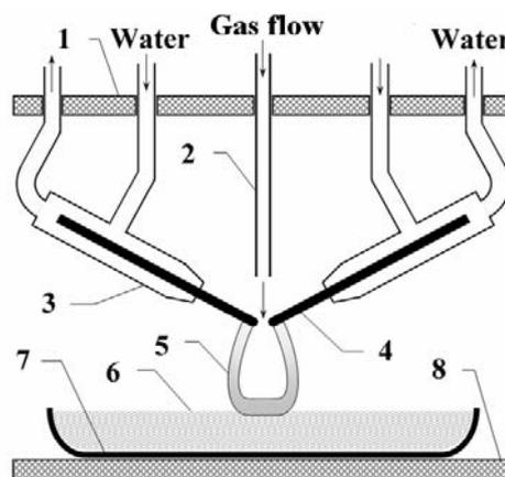
Fig.1. Scheme experimental device to study the properties of the plasma-liquid system based on secondary discharge stimulated by plasma of transverse arc.
