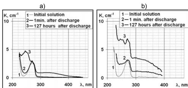
Fig.7. Evolution of phenol-water solutions after plasma assisted destruction of phenol molecules. Chart -a) correspond to secondary discharge stimulated by transverse arc with air flow; chart -b) – with
