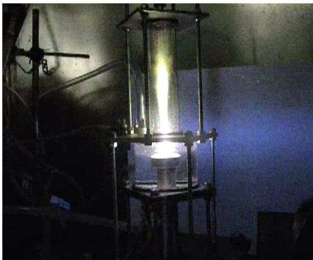
Fig.5. Photo of the PLS reactor with the DC discharge in a reverse vortex gas flow of tornado type with a "liquid" electrode during work. The gas flow  $G = 55 \text{ cm}^3/\text{s}$ . Discharge current  $I_0 = 300 \text{ mA}$ .
