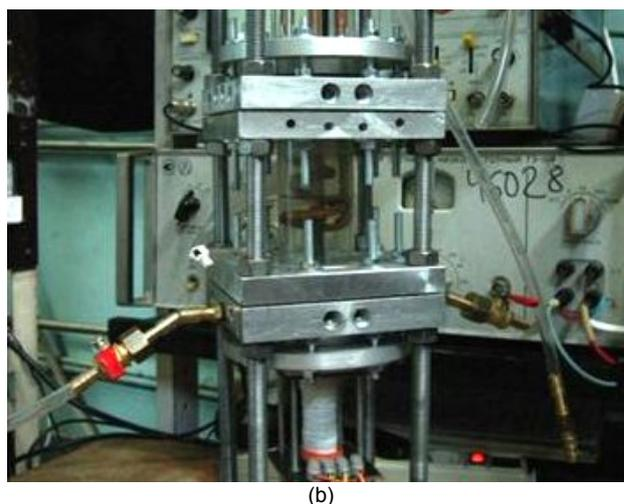
Fig.3. Scheme (a) and photo (b) of the experimental installation for studying a plasma-liquid system based on the DC discharge in the gas channel with liquid wall and the additional excitation of ultrasonic field in liquid.
