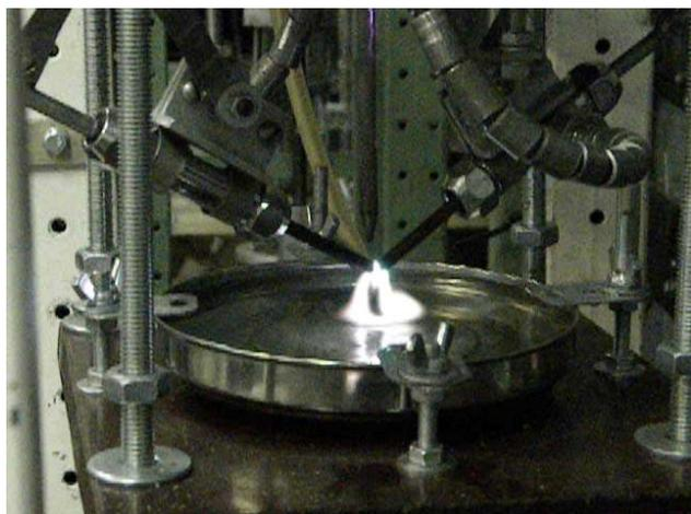
Fig.2. Photo of the plasma-liquid system based on secondary discharge stimulated by plasma of transverse arc during work.
