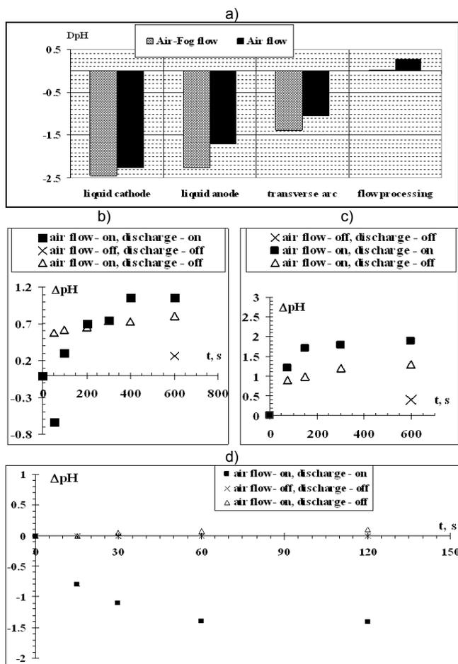
Fig.6. Variation of pH value from airflow with and without plasma treatment. a) - PLS with secondary discharge; b), c) - with DC and Pulse discharges in the gas channel with liquid wall; d) - with the discharge in reverse-vortex gas flow of "tornado" type with liquid electrode.
