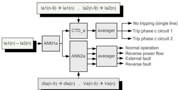
Fig. 3. Inputs and outputs of phase (a) protective modules
