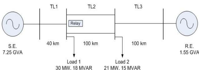
Fig. 1. Single-line diagram for power system model.
