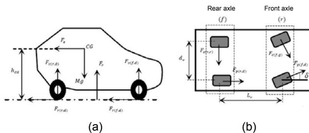
Fig.6 Lateral view (a) from below (b) different forces applied to vehicle
