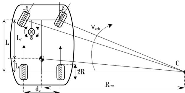
Fig.9 Vehicle structure in a turn
