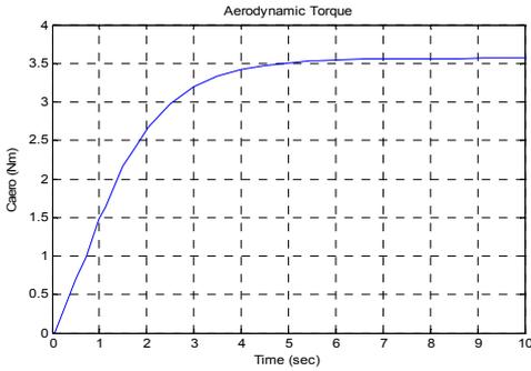
Fig.11 Aerodynamic torque  $V_{veh}=20\text{km/h}$
