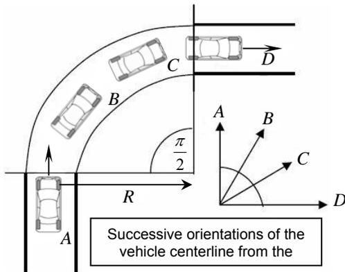
Fig.8 Yaw rate of the vehicle when taking a turn
