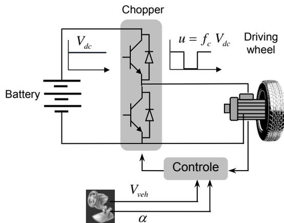
Fig.7 Control structure of the traction chain of a driving wheel with buck chopper
