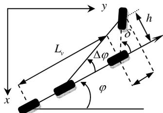
Fig.4 Kinematic model of the vehicle
