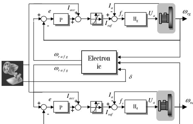
Fig.1 Two driving wheels traction chain structure
