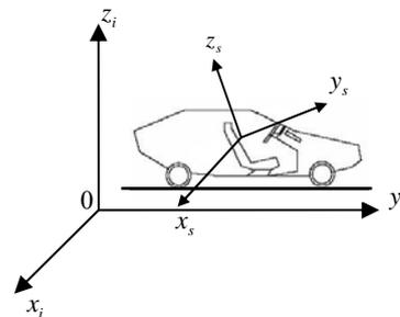
Fig.2 Presentation of the Vehicle in the Cartesian Frame
