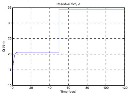
Fig.14 Resistive torque to overcome for traction
