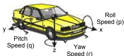
Fig.5 Variables of motion and speeds of the vehicle attached to the axis system
