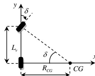
Fig.3 Bicycle model in the inertial frame
