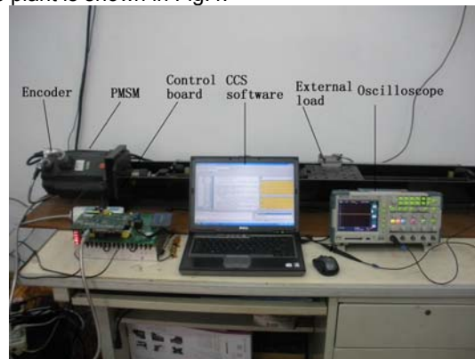
Fig.4. Plant of the PMSM servo drive
