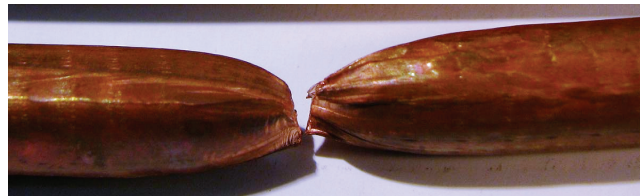
Fig. 8. DCC-AGH® wire rod after tensile test
