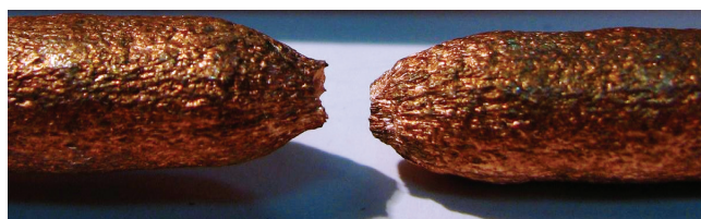
Fig. 7. Upcast® wire rod after tensile test
