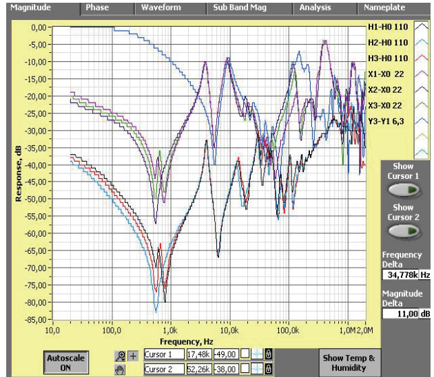
Fig.8 Magnitude Chart of three-winding transformer (primary, secondary and tertiary windings)
