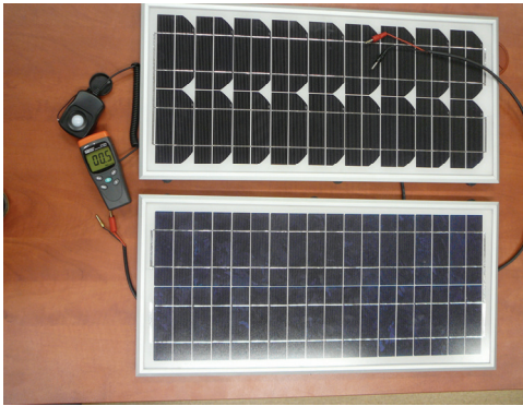
Fig. 3. The tested monocrystalline and polycrystalline photovoltaic modules SUNTECH STP 020-12/cb
