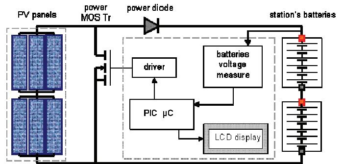
Fig. 3. Structure of the charge regulator
