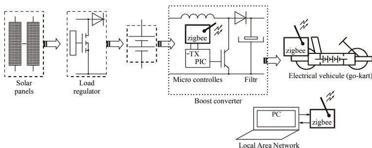
Fig. 2. Charging station principle
