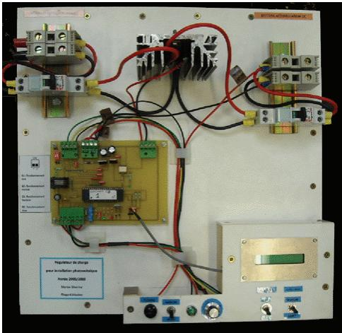
Fig. 4. Picture of the charge regulator prototype
