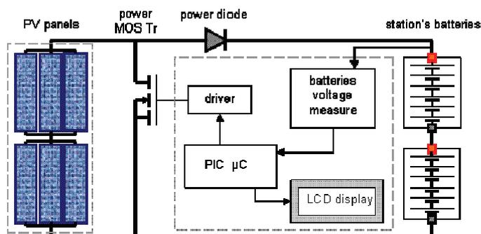
Fig. 3. Structure of the charge regulator
