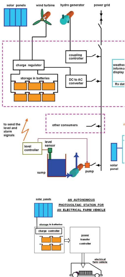
Fig. 1. General view of the electricity production and management system of an agricultural utility
