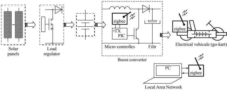
Fig. 2. Charging station principle
