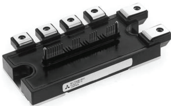
Fig. 13. Intelligent power modules MITSUBISHI PM75CL1A120: 3-phase, 75A, 1200V, current-sense and temperature sense IGBT type inverter
