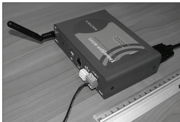
Fig.4. Main controller for MD – Moxa ThinkCore W345
