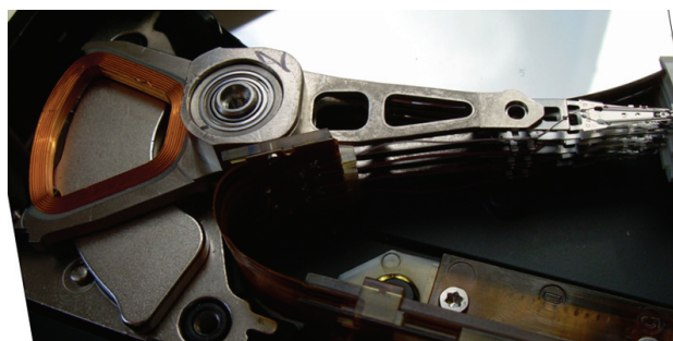
Fig.3. The head positioning system working with areal densities up to 15 \text{ Gb/in}^2
