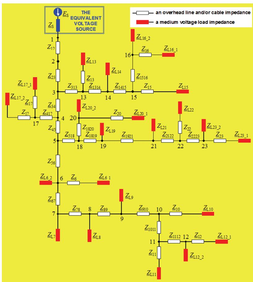
Fig. 1. Topological segment of the analyzed medium voltage(MV) power grid
