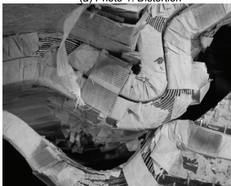
(b) Photo 2: Bulge
