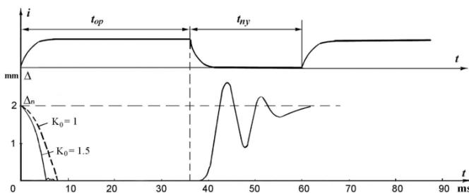
Fig. 7. Current ( $i$ ) in driving coil and displacement ( $t$ ) of the movable blade in time under closure and following releasing.
