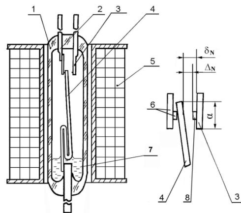
Fig. 1. Mercury wetted change-over reed switch (russian KRM-7 type) glass envelope; 2,3,4-blades; 5-driving coil; 6,8-contact elements; 7-mercury;
