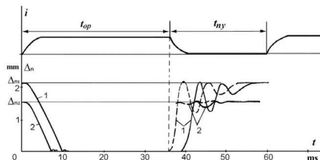
Fig. 9. Current ( $i$ ) in driving coil and displacement ( $t$ ) of the blade in time for two ( $\Delta_{n1}$ ,  $\Delta_{n2}$ ) contact gap values with (solid line) and without (dashed line) diode applied to the energizing coil ( $K_o=1.5$ )
