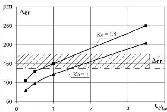
Fig. 2. Variation of critical contact gap value ( $\Delta_{cr}$ ) with time duration  $t_{ny}$  of energizing stoppage (driving voltage pulse width  $t_{op}=20\text{ms}$ ) and overdriving factor  $K_o$  value ( $\Delta'_{cr}$  for quasi steady state operation)
