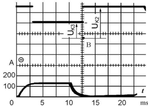
Fig. 4. Oscillograph records of voltage across break ( $U_{k2}$ ) and make ( $U_{k3}$ ) contact respectively and variation of energizing MMF ( $\Theta$ ) with time during spontaneous (single) operation of the change-over mercury wetted reed switch
