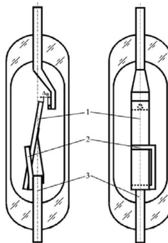
Fig. 8. Mercury wetted make reed structure with a movement limiter (support) of the movable blade, (1-movable blade, 2-nonmagnetic, electroconducting, movement limiter (support), 3-filling pipe.)
