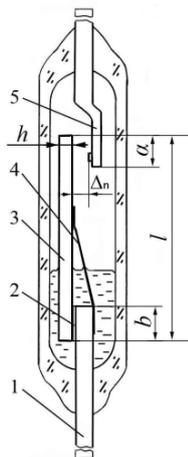
Fig. 6. Mercury wetted make reed switch with nonmagnetic pad 1-pumping tube, 2-nonmagnetic ( electroconducting) pad, 3- movable blade, 4- return spring, 5-stationary blade. ( $l=21\text{mm}$ ,  $h=0.6\text{mm}$ ,  $\alpha=2.2\text{mm}$ ,  $b=1.4\text{mm}$ ,  $\Delta_n=2\text{mm}$ ,  $\Theta=400\text{A}$ )
