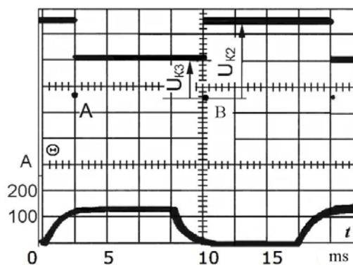
Fig. 5. Oscillograph records for the same mercury wetted reed switch but operated continuously with frequency of 50Hz.
