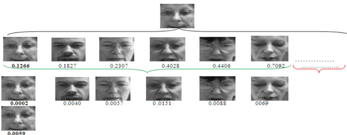
Fig. 6: Case-II: first row contain probe image, 2nd row contains the Euclidian distance computed on LDA, and row 3 contains CSLDA weights on small dataset, whereas row 4 contain new results after fusion.
