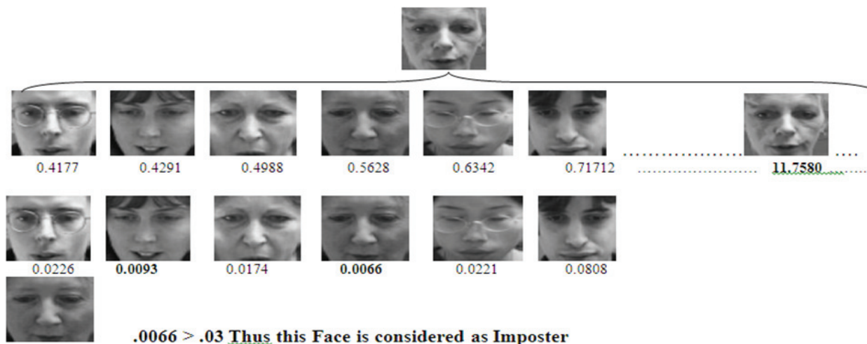
Fig. 7: Case-III: first row contain probe image, 2nd row contains the Euclidian distance computed on LDA, and row 3 contains CSLDA weights on small dataset, whereas row 4 contain new results after fusion.
