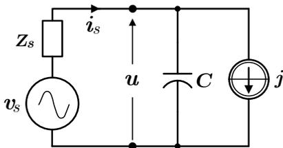
Fig. 3. Equivalent circuit of compensated load for  $\omega \gg \omega_1$ , where a current source  $j$  represents the harmonics generated by the load and  $Z_s = j\omega L_s$  is the inductive impedance of the source.
