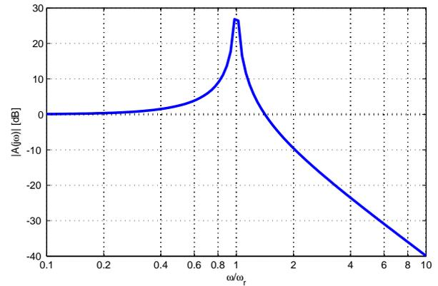
Fig. 4. Bode plot of L/DV transmittance versus relative frequency  $\omega/\omega_r$
