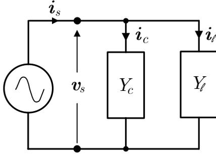
Fig. 2. Schematic diagram of shunt PF compensation configuration.
