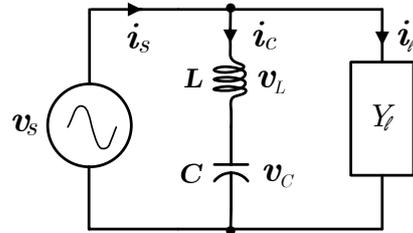
Fig. 5. Series LC-Compensation of Linear Network.
