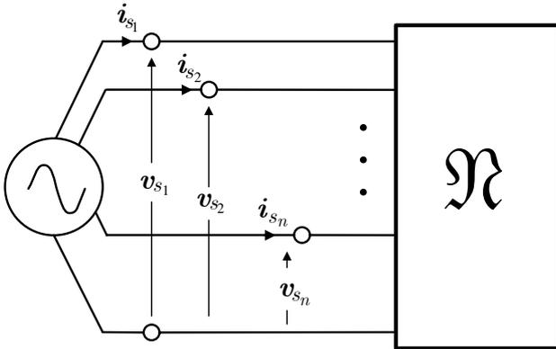
Fig. 1. Illustrating power delivered to a (possibly nonlinear and time varying) load from an  $n$ -phase ac ideal generator.
